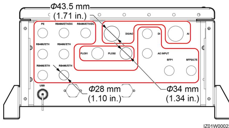
**Step 1** Remove the locking cap and plug from the waterproof connector, and then remove the waterproof connector.
