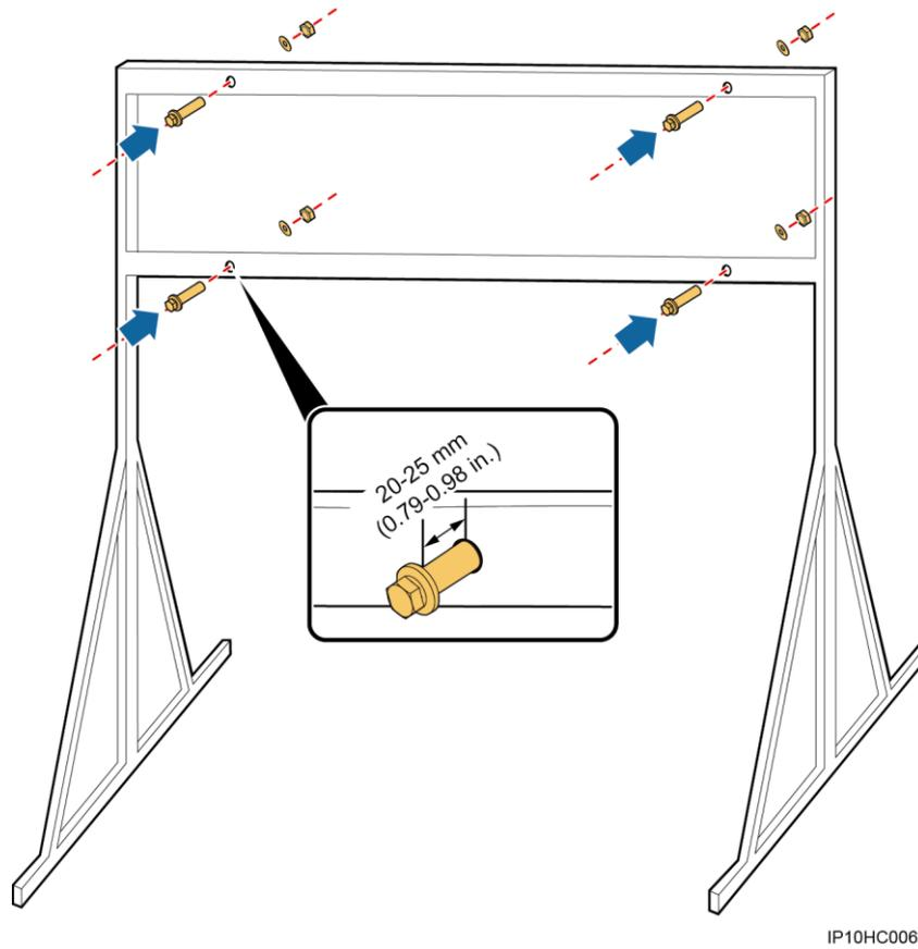
**Step 4** Assign two persons to lift the cabinet and mount it onto the bolts, and assign another person to assist.
