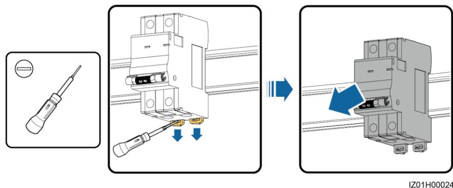
**Step 3** Install the new single-phase input switch.
