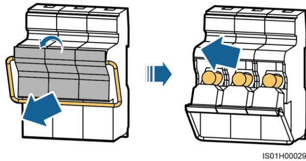
**Step 3** Install the new fuse and close the knife fuse switch box.
