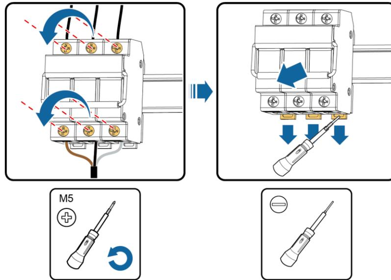
**Step 3** Install the new three-phase input switch.
