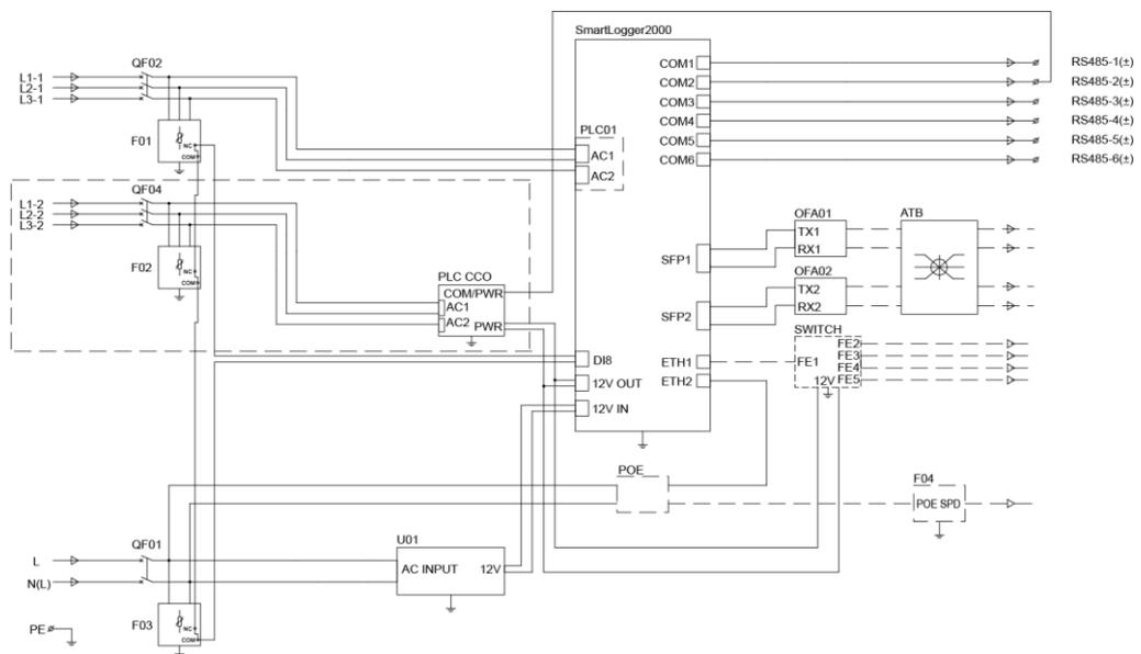
**Figure 2-9** Electrical conceptual diagram (for the smart array controller not supporting 24 V DC input or output with FU01 knife switch)
