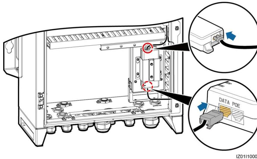
**Step 3** Connect the CPE network cable to the POE port on the POE module.
