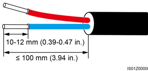
**Step 2** Connect the 24 V DC output power cable to the JX02 terminal block.
