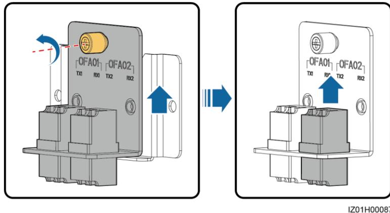
**Step 3** Install the new fiber adapter on the fastener.
